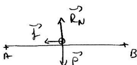
$$1b \quad W(\vec{R}_N) = \vec{R}_N \cdot \vec{AB} = 0 \quad \text{car } \vec{R}_N \perp \vec{AB}$$
